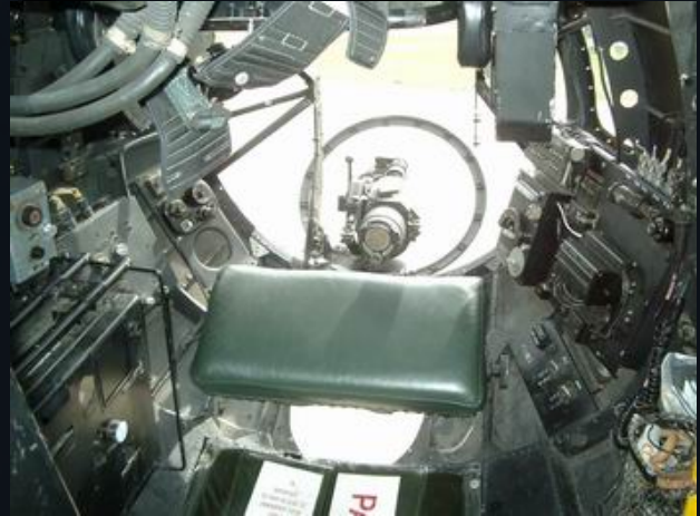
Above left: As Air Bomber, Reg takes his position in the 'chin' of the Lancaster. If called upon to do so, he would also man the forward machine gun turret. Above right: A padded bench for the Air Bomber's chest is all there is for comfort in a somewhat cramped and technology-filled space.
